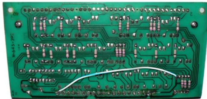
For the list of resistors to remove for your board model, see the *LIST OF COMPONENTS CHANGED PER DISPLAY MODEL* toward the end of this document. Their silkscreen markings will differ depending on the display you're working on.
