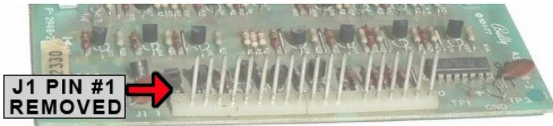
This is the high voltage pin. Failure to remove this pin will result in high voltage making its way into the 5v circuits of your machine!! **Even if you plan to remove the high voltage fuses, do not skip this step, as damage may be caused if anyone else (including you) plugs the display into a different machine that hasn't had its high voltage fuses removed.**
