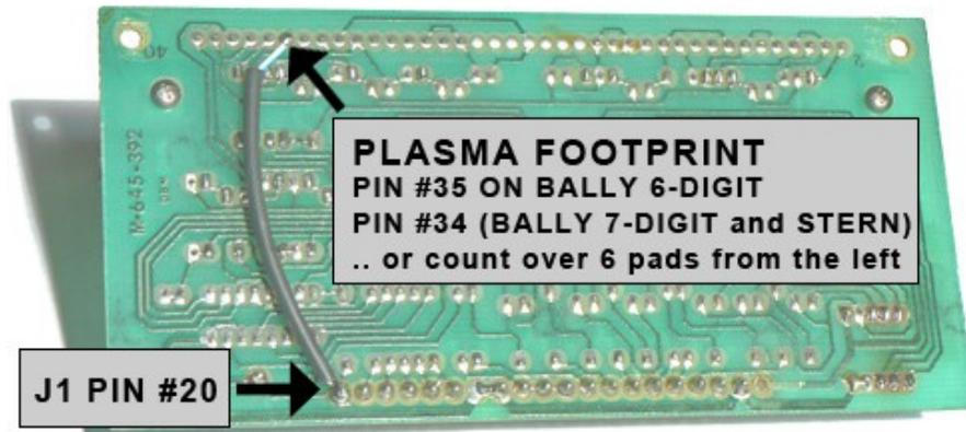
The advantage to running the jumper like this is it stays clear of the rubber supports on the mounting bracket & it's also a fairly straight shot between the two. The disadvantage is early AS-2518-15 and early "green" STERN DA100 boards do not have this pad connected. Some boards may also have other components or solder points interfere with this configuration of the jumper. Some other options are below.
