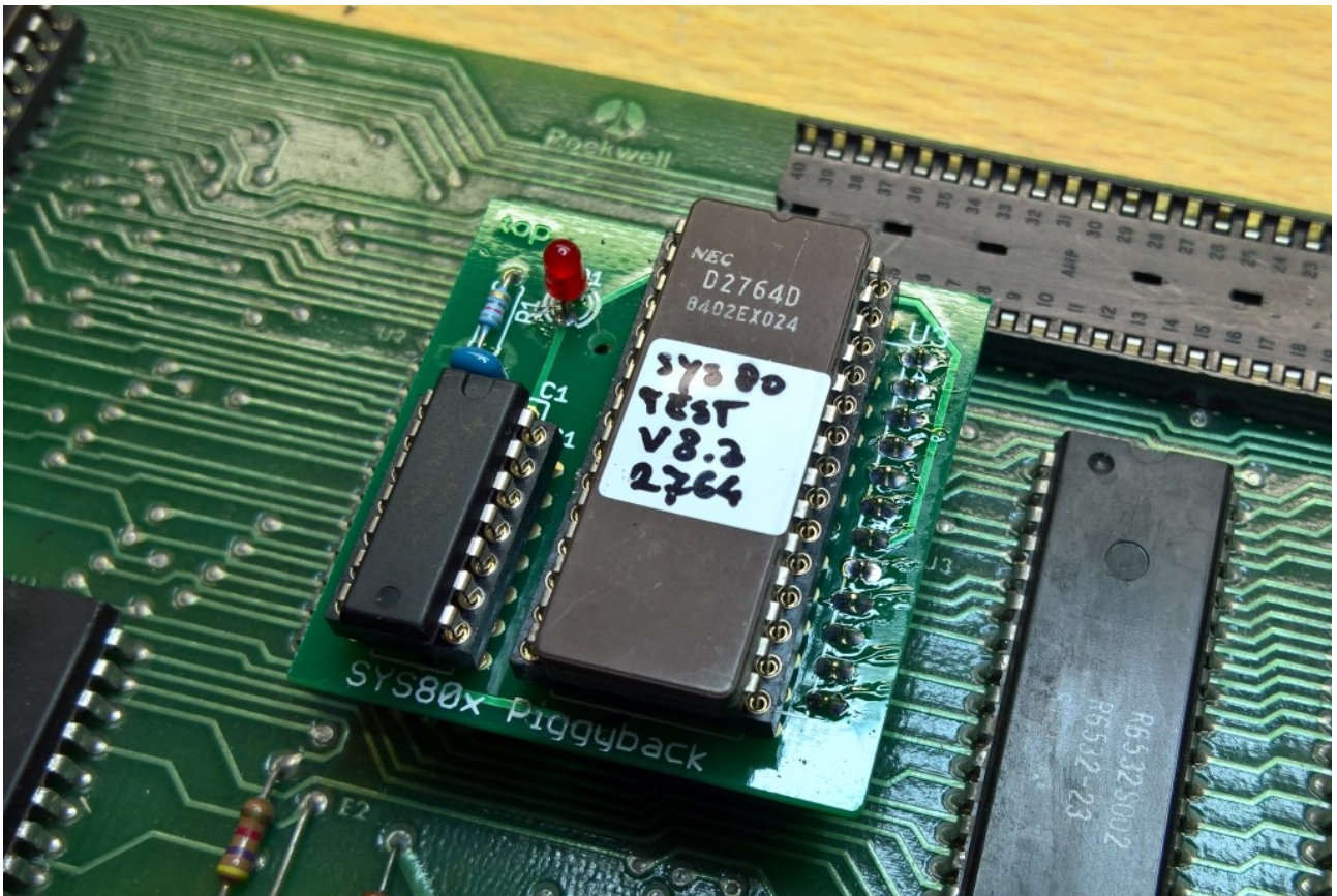
Using the testrom in a -aftermarket- Piggyback
