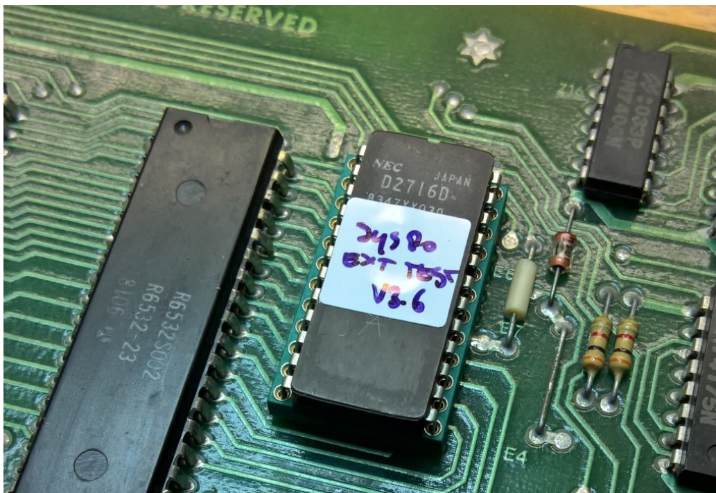
Installing Extended testrom
